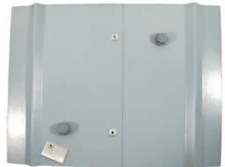
Figure 12. A Colorcoat Prisma® test panel after more than 2 years exposure
