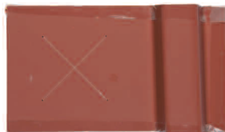
Figure 17. Test panel after humidity 1000 hrs
