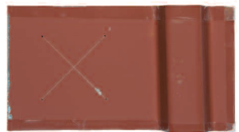
Figure 16. Test panel after prohesion 1000 hrs
