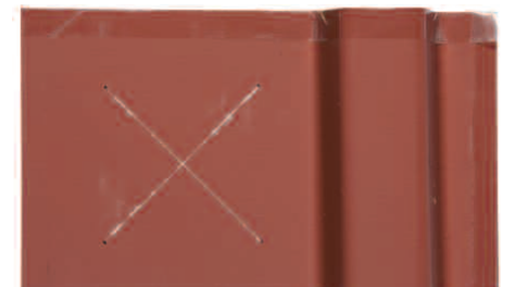
Figure 18. Test panel after water soak 1000 hrs
