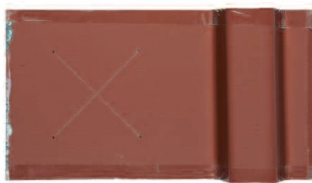
Figure 15. Test panel after saltspray 1000 hrs
