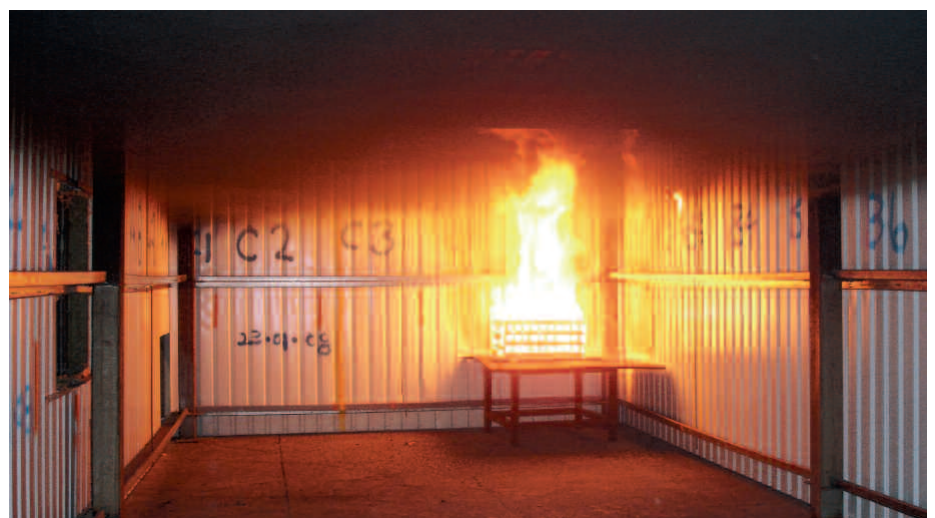
Figure 28. Example of material during an LPS 1181 test
