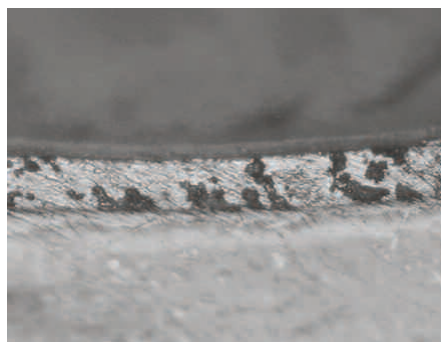
Figure 6. Galvalloy® microstructure after corrosion
